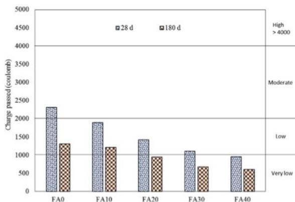
Figure 5: Effect of FA on chloride permeability
