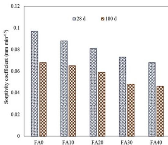
Figure 4: Effect of FA on sorptivity of concrete
